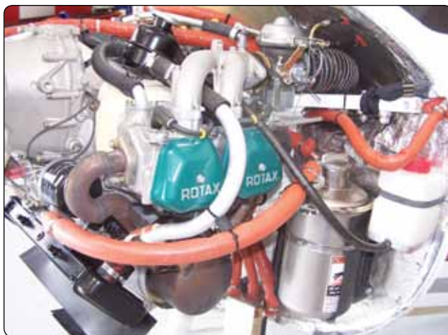
Figure 11-6. Typical four cylinder, four-stroke horizontally opposed engine.
