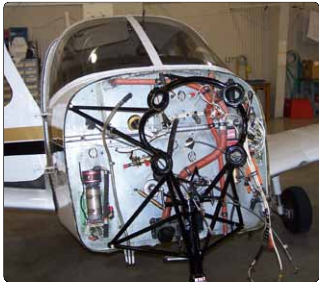
Figure 8-2. Typical firewall with components mounted on it.
