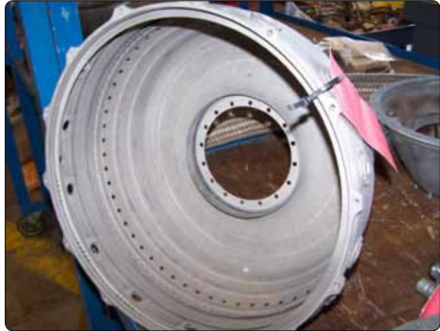
Figure 10-63. Combustion case inspection.
