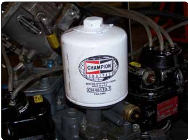
Figure 6-8. Full flow spin-on filter.
