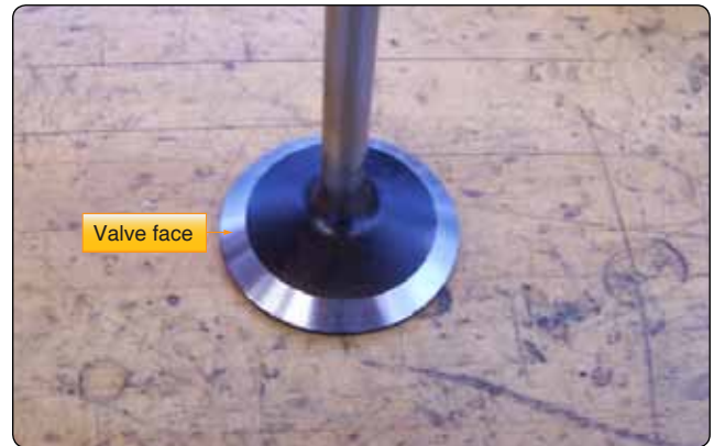
Figure 10-15. Valve face surface.
