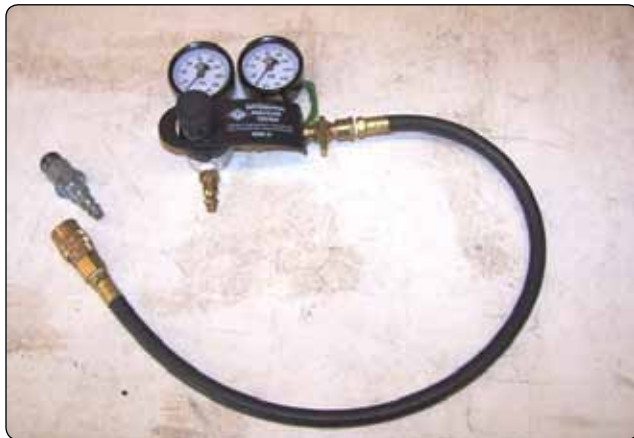
Figure 10-54. Compression tester and adapter.
