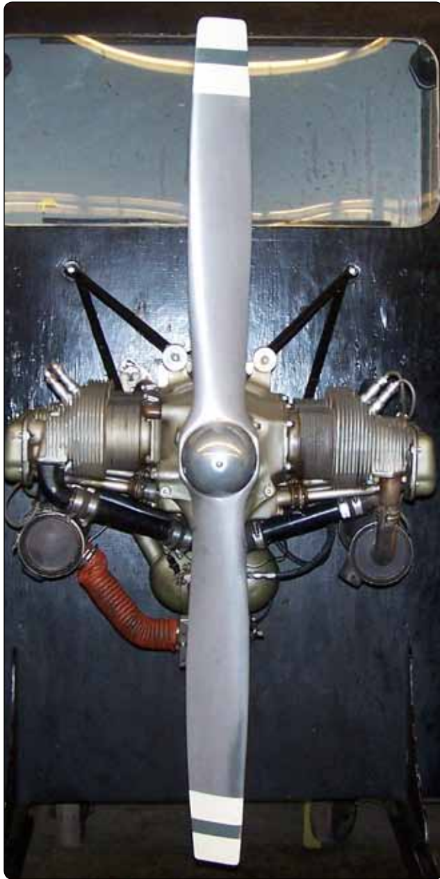
Figure 7-11. Fixed-pitch propeller.
