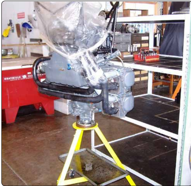
Figure 10-1. Engine mounted on an overhaul stand.
