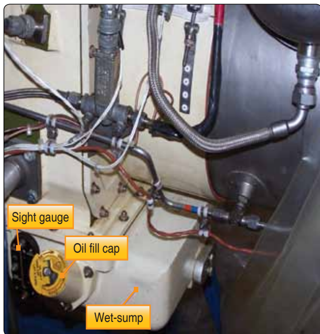
Figure 6-47. Typical turbine wet sump system.
