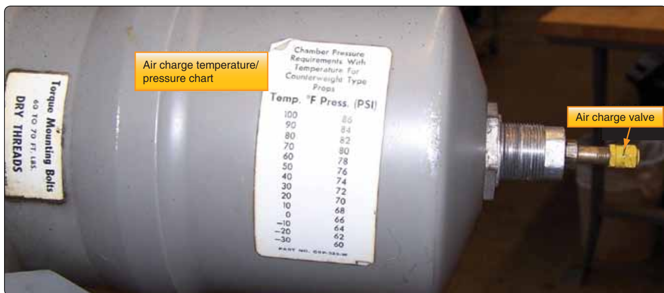
Figure 7-41. Servicing air charge in propeller.
