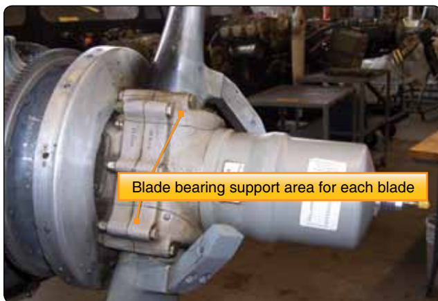
Figure 7-13. Blade bearing areas in hub.
