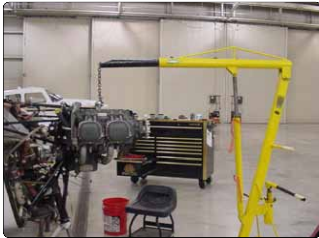
Figure 8-14. Relieve tension on engine mounts.
