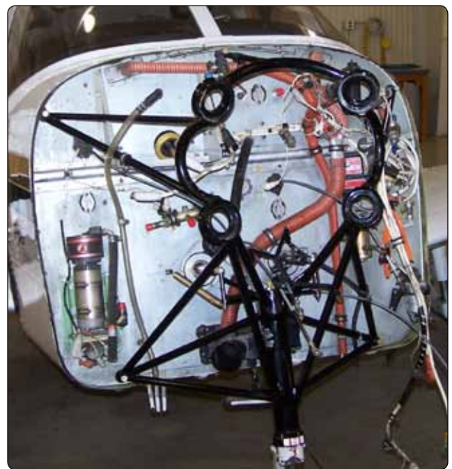
Figure 8-25. Engine mounting ring.
