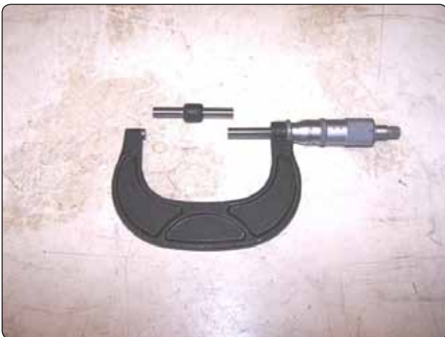
Figure 10-11. A micrometer.
