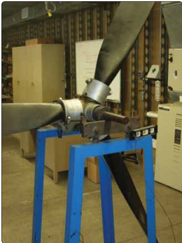
Figure 7-40. Static propeller balancing.
