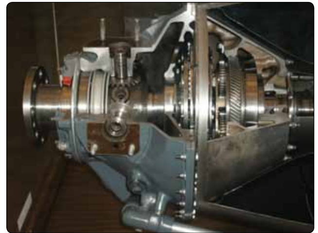
Figure 7-46. Reduction gearbox.
