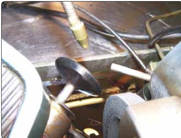
Figure 10-25. Valve in chuck ready to grind.
